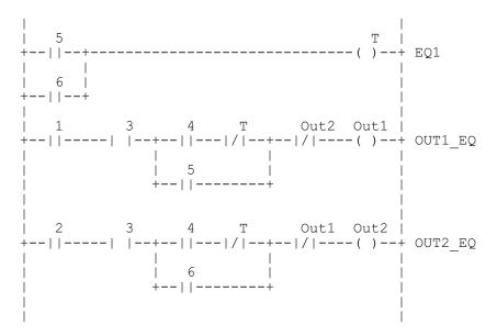
Rung T is equation 1. It is necessary because it is needed in two equations and because the equations would be 80 characters long without the semicolon.
